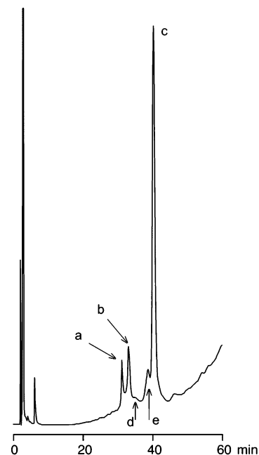
Figure 6. Air oxidation of an equimolar mixture of \alpha(1,2) -SH and \alpha(3,4) -SH ( 75 \mu\text{M} of peptide in 5 mM aqueous phosphate buffer, pH 7.1, 20^\circ\text{C} , 4 h). HPLC conditions: linear gradient from 20% to 60% B; A, \text{H}_2\text{O} + 0.045\% TFA and B, MeCN + 0.036% TFA; 1 mL/min, 220 nm. (a) \alpha(1,2) -SH, (b) \alpha(3,4) -SH, (c) \alpha(1,2)\text{-S-S-}\alpha(3,4) , (d) \alpha(1,2)\text{-S-S-}\alpha(1,2) , and (e) \alpha(3,4)\text{-S-S-}\alpha(3,4) .
